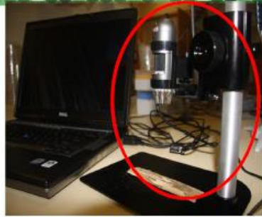
Dinolite – see the magnified image in the field or lab
